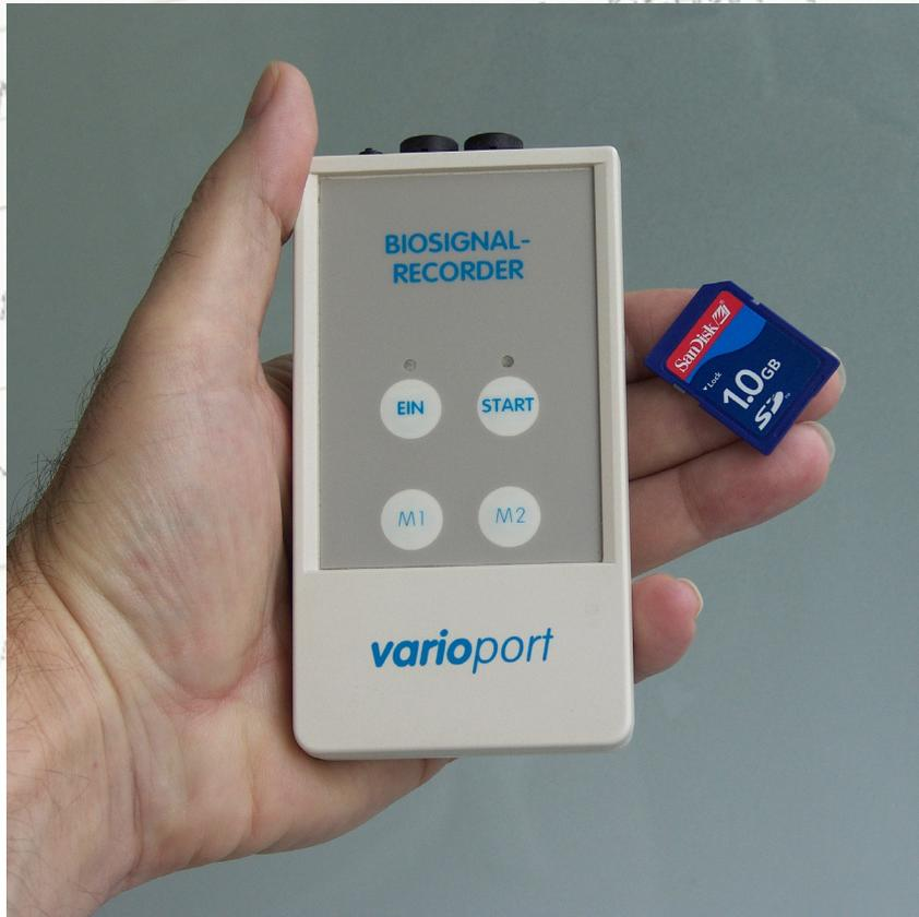
*The varioport recorder system is a very small and lightweight portable measuring system. It collects physiological, movement and environmental data over a time period up to one week.*
